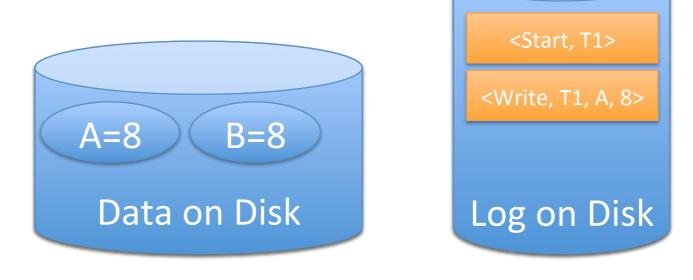
T1: Read (A, t); t <-- t x 2; Write(A, t); Read (B, t); t <-- t x 2; Write(B, t);
