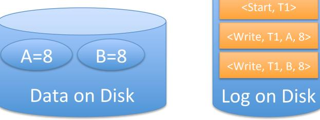
T1: Read (A, t); t <-- t x 2; Write(A, t); Read (B, t); t <-- t x 2; Write(B, t);
