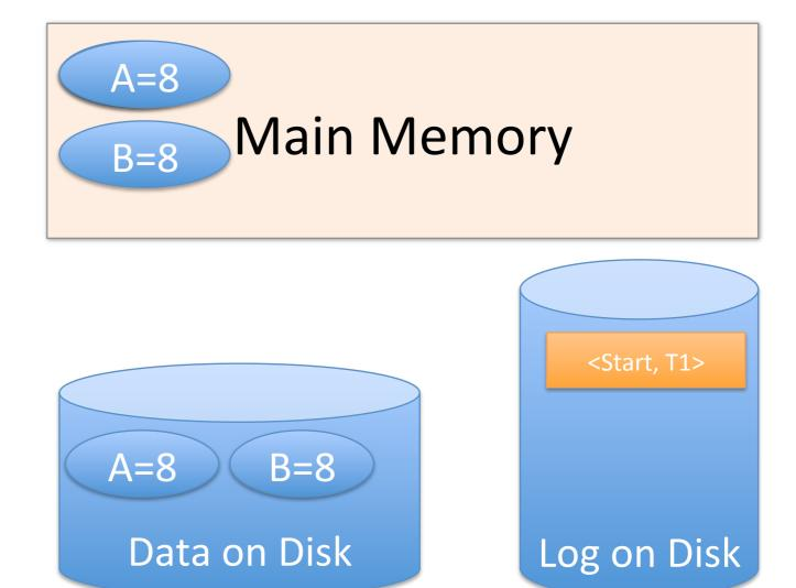
T1: Read (A, t); t <-- t x 2; Write(A, t); Read (B, t); t <-- t x 2; Write(B, t);
