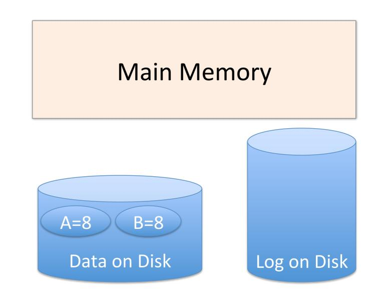
T1: Read (A, t); t <-- t x 2; Write(A, t); Read (B, t); t <-- t x 2; Write(B, t);
